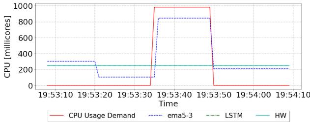
Fig. 7. Cold starts for HW and LSTM compared to ema5-3 when running image\_rotate\_shorter workload. Due to lack of historical information and training, LSTM and HW cannot allocate sufficient CPU. LSTM and HW curves overlap.
